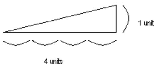
2. **Degrees** - this is a measurement used to represent the angle of a slope. Degrees can be measured with a protractor or with survey instruments. Land that is completely flat (horizontal) is  $0^\circ$ , while a vertical cliff is  $90^\circ$ .
