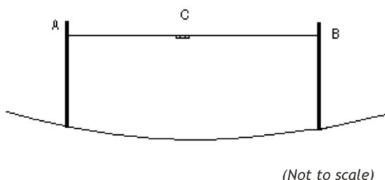
Start at the edge of the field. Person A holds their pole in a vertical position and stands still, while person B moves up and/or down the slope until the line level, which is read by person C, gives a level reading. Points A and B are then marked with pegs.
