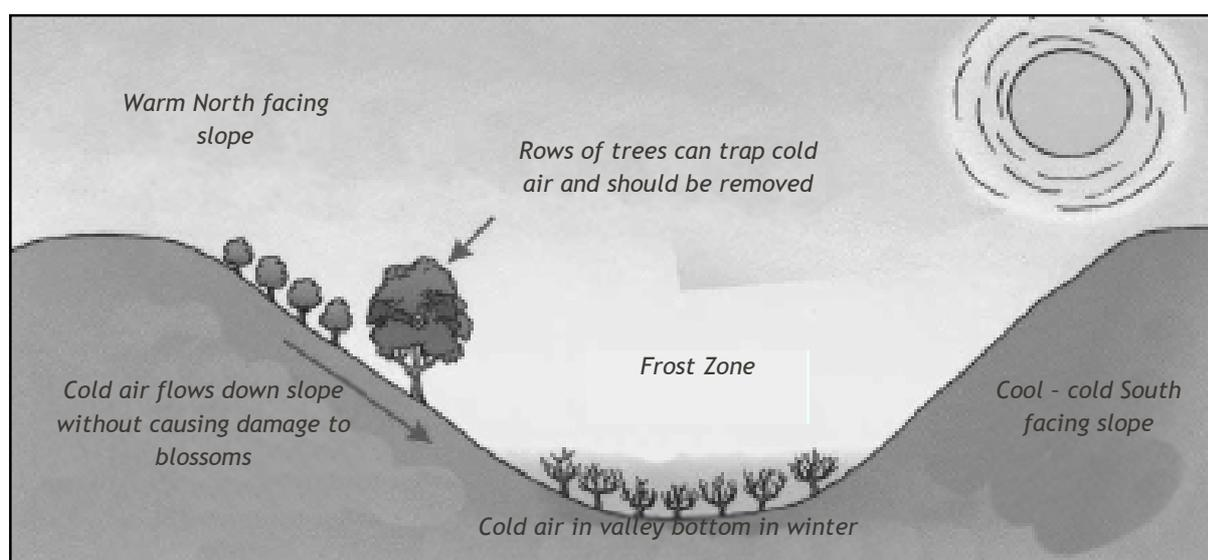
Figure 16.1: Diagram of different zones
