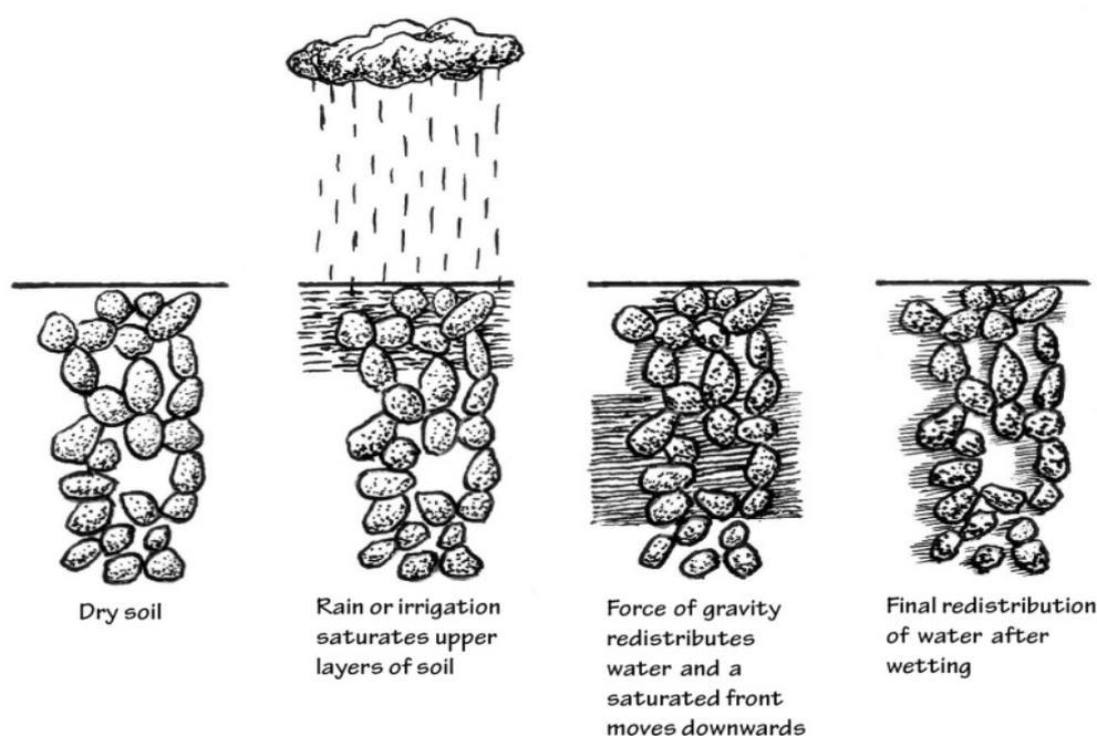
Figure 5.3: Water in the soil
