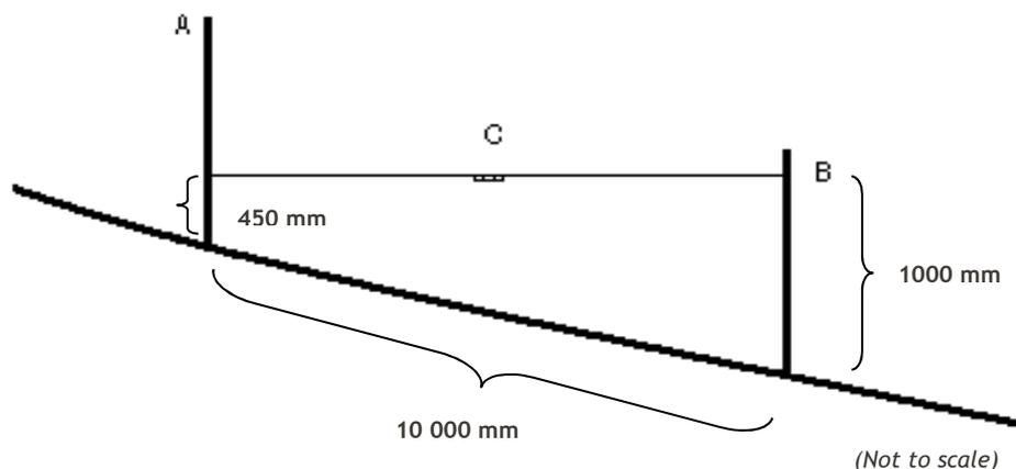
Figure 2.5: Using a line level to measure slope
