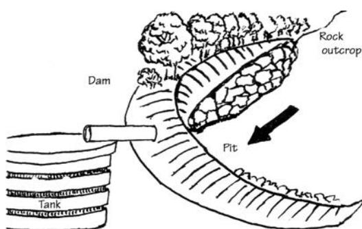
Figure 1.5: Water overflow is directed into a storage tank
